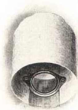
View of lower end of heater showing frame for holding mica, with small sheet of isinglass partly removed. See "Latest Heater Improvements," on page 17.
